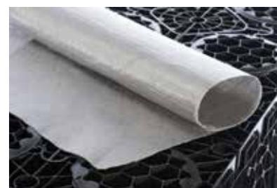
A polypropylene permeable non-woven geotextile, for use in infiltration applications. ACOTex permits the passage of water into and out of ACO StormBrixx system, and also prevents the entry of sediment into tanks incorporating sediment forebays.
