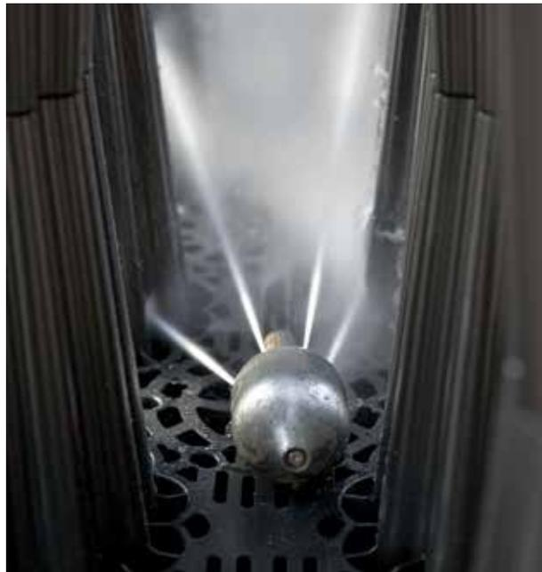
Cleaning equipment with a rinsing head. Any deposits that may be in the system can be pressure-rinsed and suctioned at the same time.
