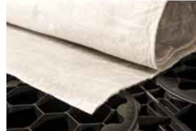
Manufactured from polypropylene this thick non-woven protection fleece is used to protect a geomembrane from mechanical damage due to ground and thermal movement. The protection fleece is placed on the outer side of the geomembrane. ACOTex Plus can be used with ACOWrap or with a welded geomembrane system.
